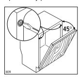
For this purpose use the two front screws. Open the door, remove the caps and screw or unscrew the screws.
